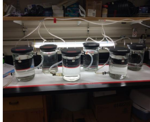
Figure 2. Experimental system with beakers bubbled with control (400 ppm) or treatment (2,500 ppm) CO 2 .
